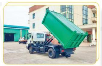
"The type of garbage truck with a hooklift system structure serves to transport waste by a tank that can be separated from the hooklift vehicle. Specializing in transporting garbage and waste, the Hooklift truck is truly a leading vehicle in the field of waste transportation."
